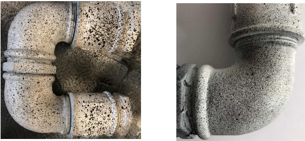
Figure 8. The surface preparation of the U pipe rough spray (left) and the fine spray (right)
